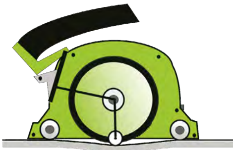
Principle of automatic depth control
